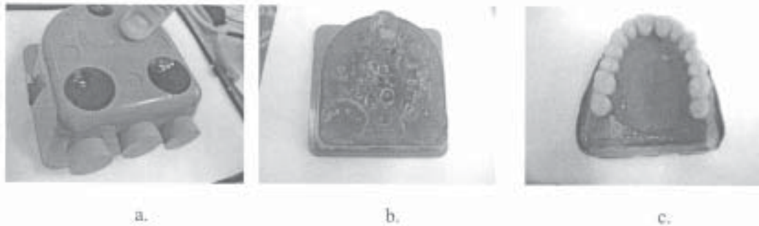
Fig. 6. Deficiencies in using reversible hydrocolloids for wax pattern investment; a. bubbles that develop in the mass of the reversible hydrocolloid in the flask; b. pressing the flask leads the development of holes in the mass of the hydrocolloid; c. melting of denture base wax.
